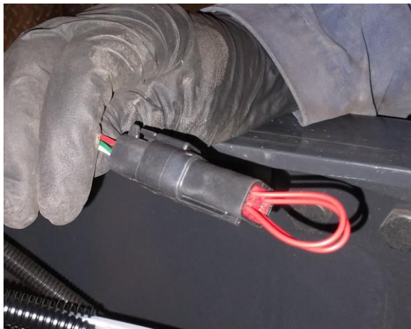
Fig 3. Install test plug
