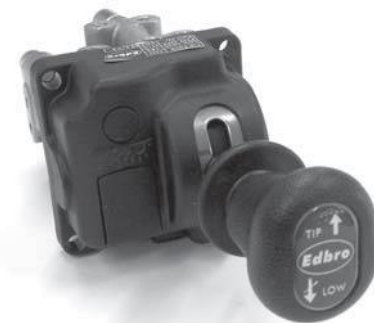
Fig. b. Separate tipper air control
